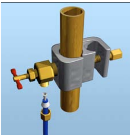
Figure 8. Connect \frac{3}{8} " valve and tubing as shown (color coding of tubing is for installation purposes)
