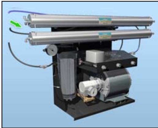
Figure 19: a) disconnect the tubing from both the RO Modules b) Remove the RO Modules from the clamps holding them to the frame
