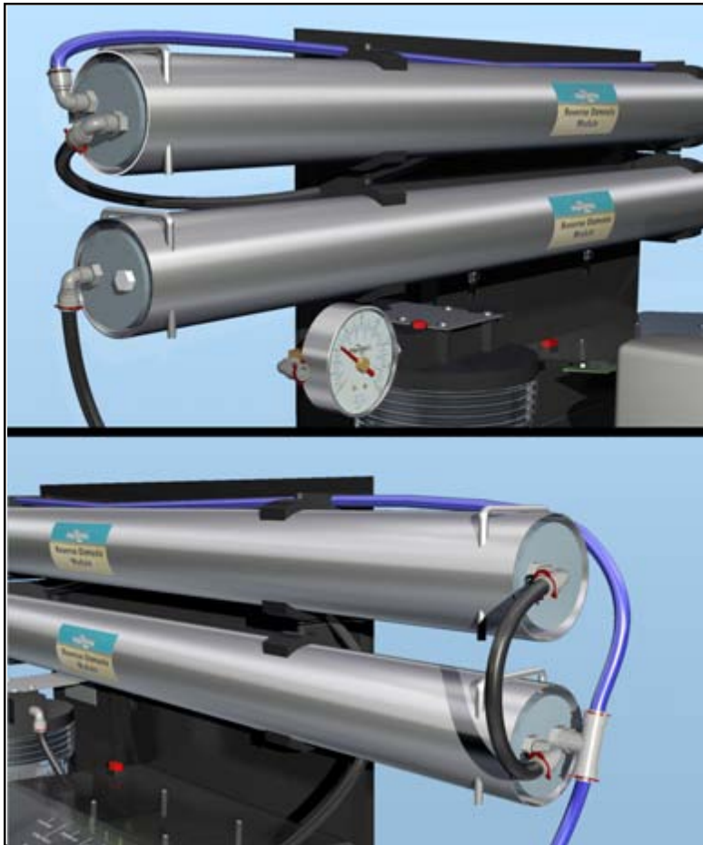
Figure 21: i) Lower RO Module has an elbow connector on one end; on the other end there is a swivel tee connector and an elbow connector ii) Upper RO Module has two swivel elbow connectors on one end and an elbow connector on the other end iii) The labels on the RO Modules should face you
