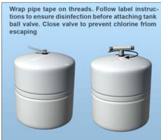
Figure 10. Storage tank preparation
