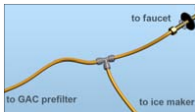
Figure 12. Connect the Ice Maker as shown (color of tubing is for illustrative purposes)
