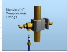
Figure 4. Feed water saddle valve.
