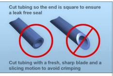
Figure 10. Cut tubing square; do not use scissors
