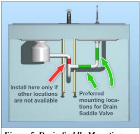
Figure 5. Drain Saddle Mounting Locations
