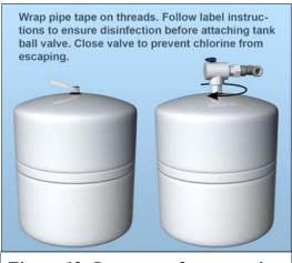
into the opening. Figure 12. Storage tank preparation
