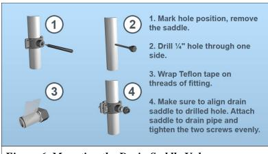
Figure 6. Mounting the Drain Saddle Valve
