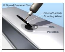
Figure 3. Using a Dremmel Tool to remove porcelain
