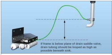
Figure 11. Drain line connection (color of tubing is for illustrative purposes)
