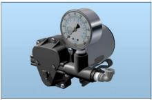
Fig. D4: Connect pressure gauge to pump
