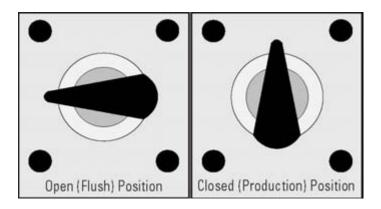
Figure 2. Front Mounted Flush Valve
