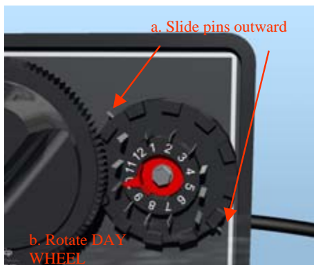
Fig. 20. (a) slide pins for day 6 and 12 outwards (ensure the others are retracted) (b) the pin (or tab) at the red pointer indicates “today”.
