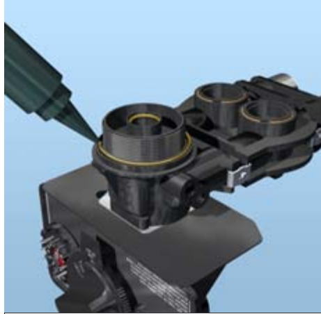
Fig. 3. Lubricate the tank o-ring.
