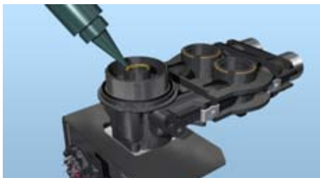
Fig. 2. Lubricate distributor o-ring with silicone lubricant.
